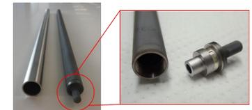
End plug sealing structure
