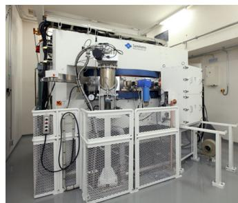
200uA  $\text{He}^{2+}$  beam will be installed at CANMT in mid-2026.
