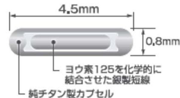
^{125}\text{I} \Phi 0.8\text{mm} / L4.5mm
