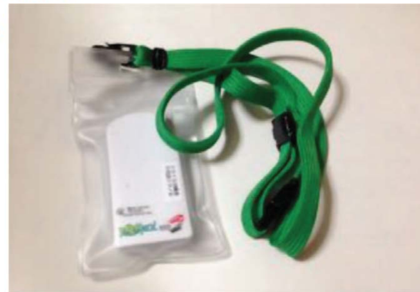
Figure 6. A semiconductor-type personal dosimeter ‘D-shuttle’, developed jointly by AIST and Chiyoda Technol Corporation. Each participant was instructed to wear the dosimeter on their chest, using the provided strap.
