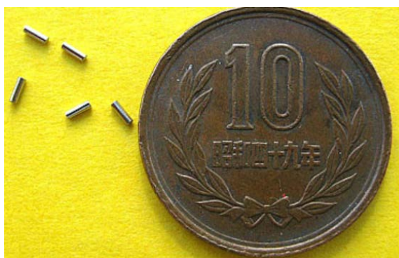
^{198}\text{Au} \Phi 0.8\text{mm} / L2.5mm
