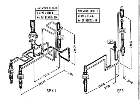
Fig. 1 Comparison of the secondary sodium loops
