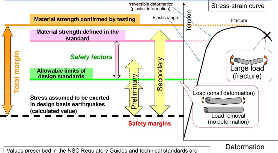
used as allowable limits in preliminary assessment. Values exceeding allowable limits are applicable if it is technically verified in the preliminary assessment that the structure's integrity and functions are maintained. Factual assessment is conducted during secondary assessment to obtain values that cause the loss of structural integrity and functions.
